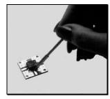
Step 2: Mount components onto ProtoCell circuit boards
